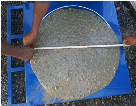
Workability measurement through Flow Table test (IS 9103)
