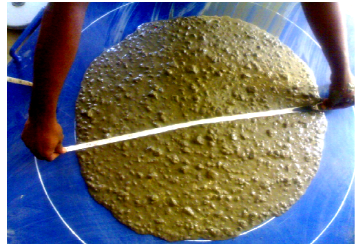
Self Compacting Concrete – Slump Flow test (European Guidelines)
