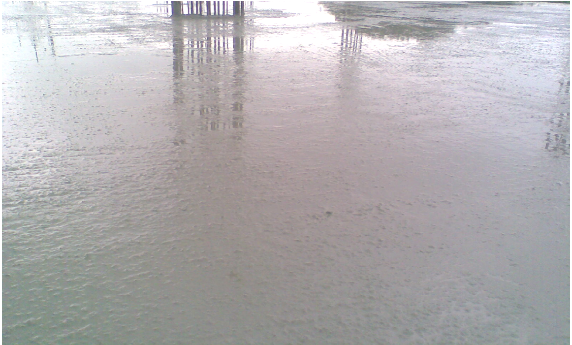
SCC fresh surface – with very little bleeding – Coarse aggregate appearing on top surface
