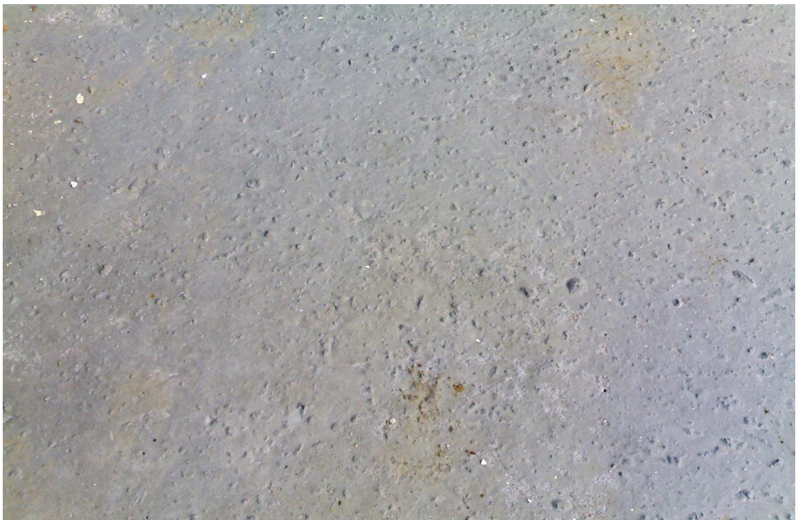
SCC hardened surface – Coarse aggregate appearing on top surface
